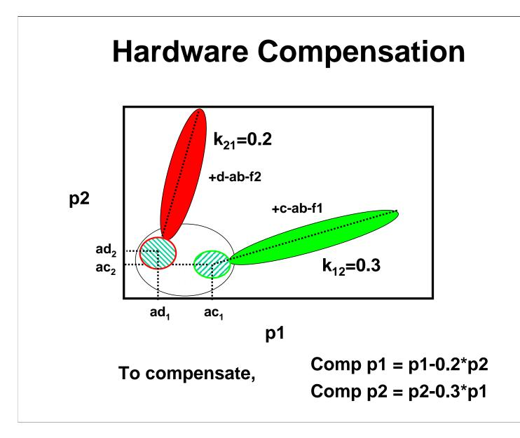
To perform hardware compensation, a certain percentage of one signal is subtracted from another. In this particular example, to exactly compensate the above signals we would subtract 20% of p2 from p1 to obtain a compensated p1 signal and 30% of p1 from p2 to compensate p2.
