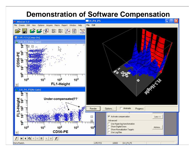
Thus, the data that appear to be under-compensated are really not. The upward trend of the upper envelope of the data is due to both counting and digital errors. Is there a better display method that avoids this under-compensated appearance?
