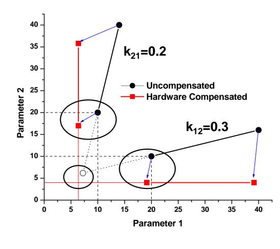
The above figure shows the geometry of our example with and without compensation. The black dots represent the autofluorescence and uncompensated fluorescence intensities for both single color controls. The red squares are the associated compensated points. Notice that the compensation results in two orthogonal lines, which is the major goal of compensation. Also note that both the autofluorescence points are shifted towards the origin (large circled areas).
