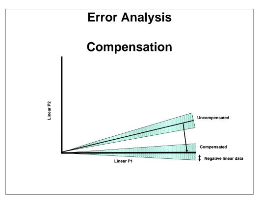
The combination of counting and digital error creates a symmetric error distribution about the single-color trace line. When this data is properly compensated, this distribution becomes symmetric about a horizontal line with some events defined below the axis. These negative values create several problems for us when we transform the axes to log.
