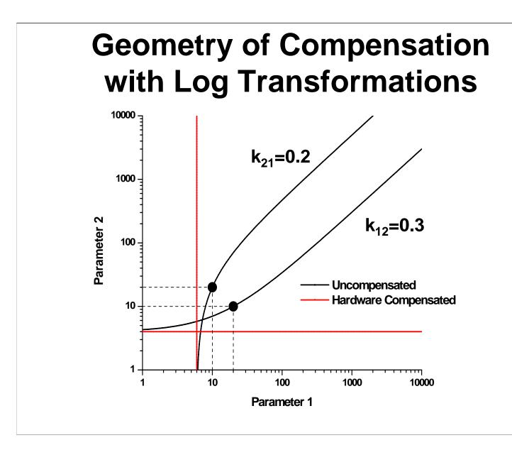
So far, we have only described and viewed the compensation process with linear parameters. What happens when we apply a four-decade log transform to both axes? The above plot is the same example we have been developing, viewed in four-log space.
