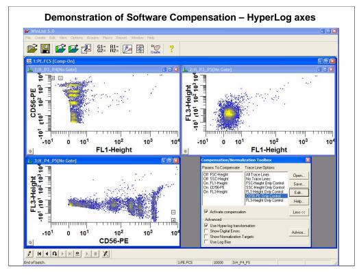
If the display axes are converted to a HyperLog scale, we can see the symmetry of the error distributions and the data appear perfectly compensated. Also, the data are no longer piled on the axes.
