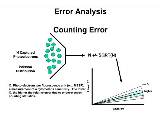
The first error we'll consider is at the level of signal detection. Since the number of photoelectrons ultimately captured by the cytometer's PMT is finite, the signal quantitation is stochastic with a variance governed by the Poisson distribution. The square-root of the number of captured photo-electrons is approximately the standard deviation of the error distribution.
