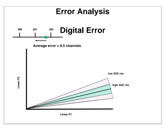
The second error we'll consider is the truncation of the analog log amplified signal to an integer value, digital error. On the average, digital error yields, on average, an error of ½ ADC channel. Unfortunately, this error is augmented by the log transform so that truncations at high ADC values can have a substantial error.
