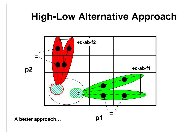
Adjust the signal subtracters such that the low and high medians for both single color populations are identical.
