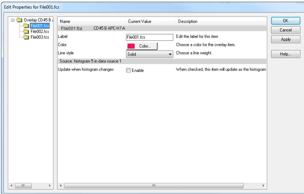
The first entry in the property list shows the source FCS file and the parameter(s) that the plot is displaying. These are not editable; they are determined at the time the item is added to the overlay.
