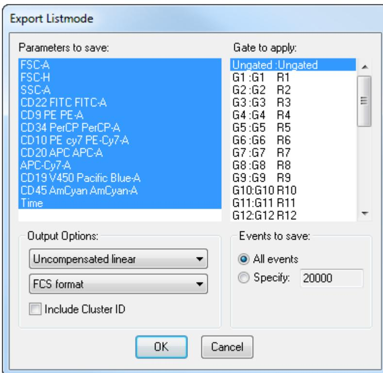
The **Parameters to save** list box shows the parameters available to save. Select parameters in this list that you want in the new listmode file.
