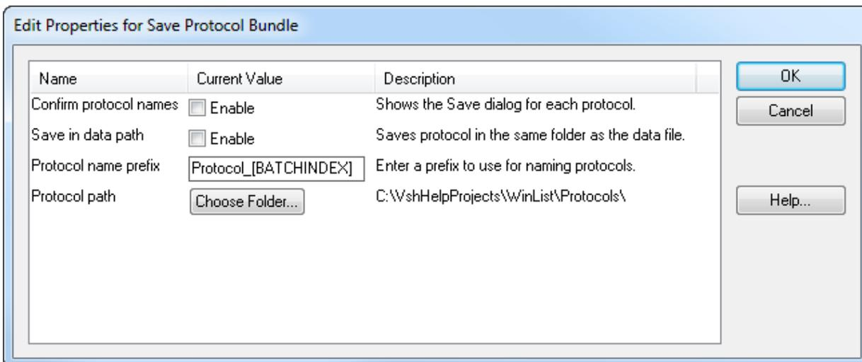
Each batch command has its own unique properties. For example, commands that relate to saving files typically have properties that allow you to set the path and file name, and commands that pause have properties that allow you to specify a prompt to display to the user.
