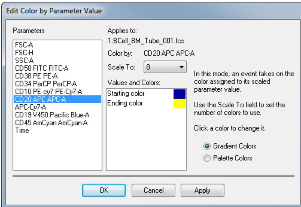
In the example below, CD20 was selected as the parameter, with dark blue representing low CD20 transitioning to yellow for high CD20. Note that the coloring appears in the CD10 vs CD45 plot to help identify the low and high intensity CD20 events.
