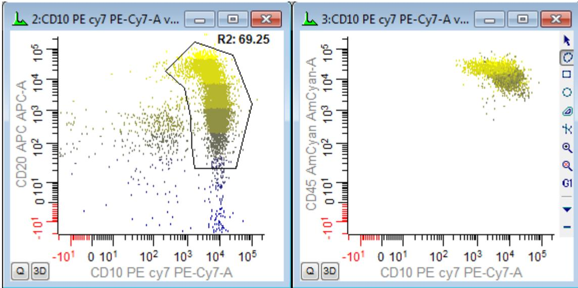
Select a parameter from the **Parameters** list. The intensity of the selected parameter will be used to color the dot for each event.
