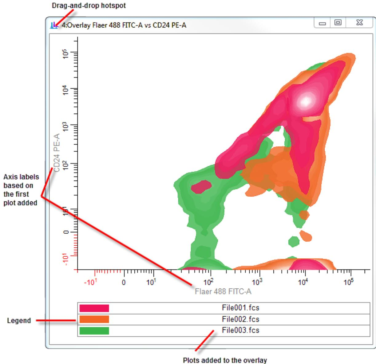
To add a plot to an overlay, drag a histogram by the icon on the left side of its toolbar and drop it onto the overlay. The first plot that is added to an overlay determines whether it is a 1P or 2P overlay window. It also determines the axes that will be displayed. If you subsequently add a plot with different parameters than the first plot, the overlay will ask if you really intend to do so.
