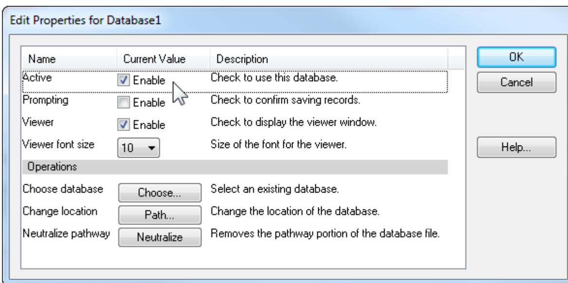
The properties are enabled or disabled with simple check boxes. Path selection is initiated by clicking the Database Path Folder button.
