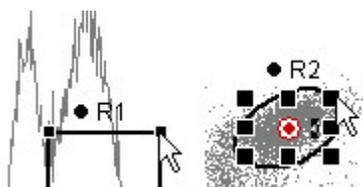
Delete a region by clicking on the region label, and then pressing the Delete key on the keyboard. You can also delete regions (except for NStat regions) by dragging the region label off the left edge of the histogram and releasing the mouse.
