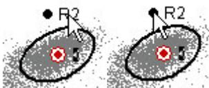
Resize a 1P or 2P region by clicking on the region's label to activate the region. Sizing handles are displayed. Click on one of the handles and drag it with the mouse to adjust the size of the region.
