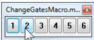
Once the Macro Toolbox is displayed, you can move it to any convenient location on the screen. Its position will be stored by WinList so that each time you run the program, the toolbox will appear where you left it.
